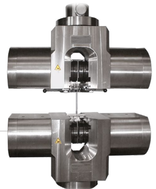
Hydraulic jaws for tensile testing at high loads
