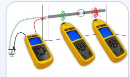
**Locate line interruptions**Quickly and easily detect breaks in your walls
