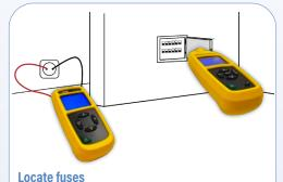
Connect the transmitter to a socket and simply find the corresponding fuse
