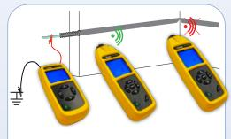
Detect the narrowed (or blocked) section of a non-metallic pipe (requires temporary insertion of a conductor)
