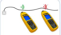
Identify the mains voltage and locate a break in the circuit
