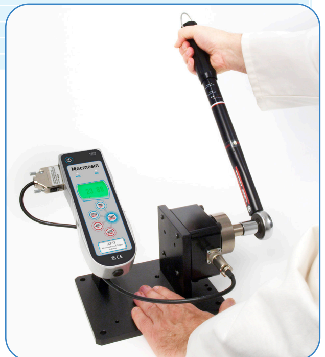
TWC shown testing a mechanical torque wrench
