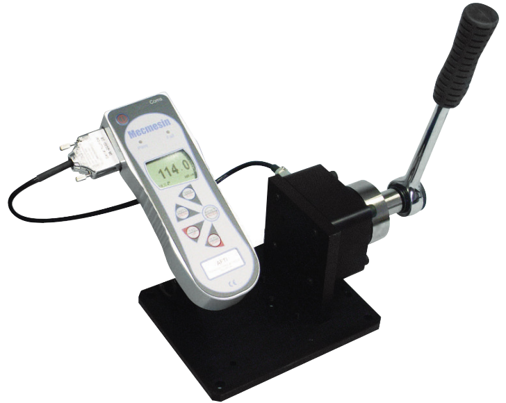
TWC shown testing a mechanical torque wrench
