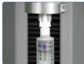
▲ Syringe cap removal
