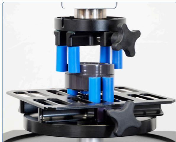
▲ Tightening torque of cosmetic container
