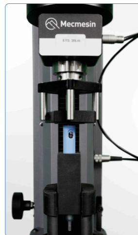
▲ Dosage torque of injector pen
