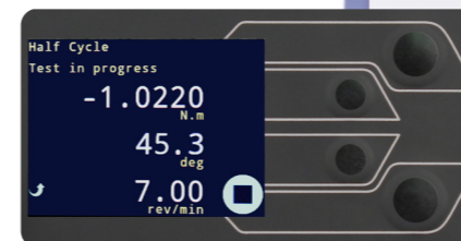
▲ Colour display of speed, angle and torque
