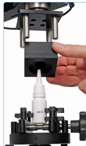
▲ Dispensing dropper testing
