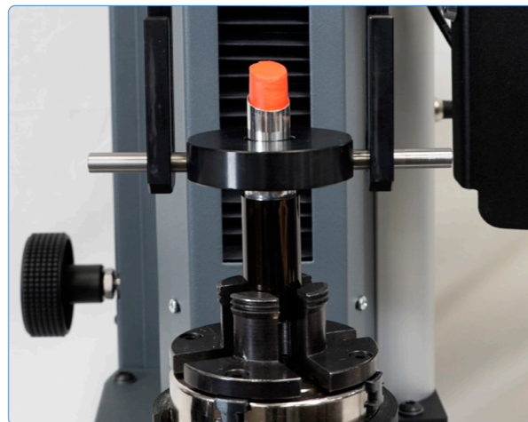
▲ Lipstick barrel rotation torque
