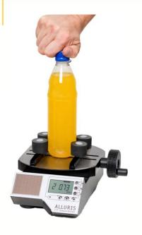
Digital Cap Torque Tester CTT-300 series with automatic detection of two peak values are designed for quick, manual torque testing of tamper evident closures. The cap is opened manually and the maximum torque for loosening the cap and for breaking the safety ring are detected separately. For both peaks limit values can be defined, which are monitored and displayed during the measurement.
