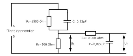
Reaction in the human body results from the current flowing within the body. The measuring circuit according to picture 4 emulates the impedance of the body and weight the reaction depended from the current causing an unwanted reaction.
