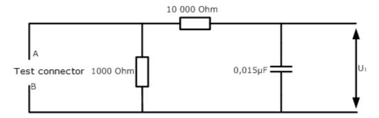
This measuring circuit corresponds to the requirement of DIN EN 60601-1:2013-12 chapter 8.7.3 part a - d.
