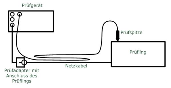
Favourable leading of the measurement wires. The aerea between the measurement cables is small keeping the appearnt resistane small.
