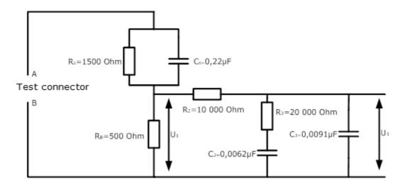
The inability to let loose the unit under test results from a current flow within the human body (e.g. through muscles). the influence of the frequency for let losse is different from the influence for reaction. this is significant for frequencies above 1 kHz.
