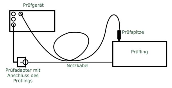
Also unfavourable leading of the measurement cables. The aerea between the measurement cables is smaller but the appearnt resistance will increase due to the loop.
