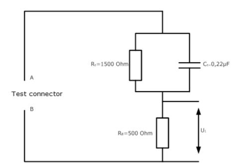
This measuring model emulates the impedance of the human body. This allows sto measure the current flowing through a human body touching the unit under test in a similar way.
