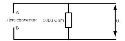
This measuring circuit corresponds to the requirement of DIN EN 60601-1:2013-12 chapter 8.7.3 part e.
