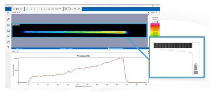
Each sensor requires its own unique MAP driver file for the software to function properly. By utilizing sensor MAPs, the software is able to provide an accurate depiction of each unique sensor layout. The sensor MAP controls the shape of the pressure image window in the software, which corresponds to the shape and dimensions of the sensing area on the sensor.
