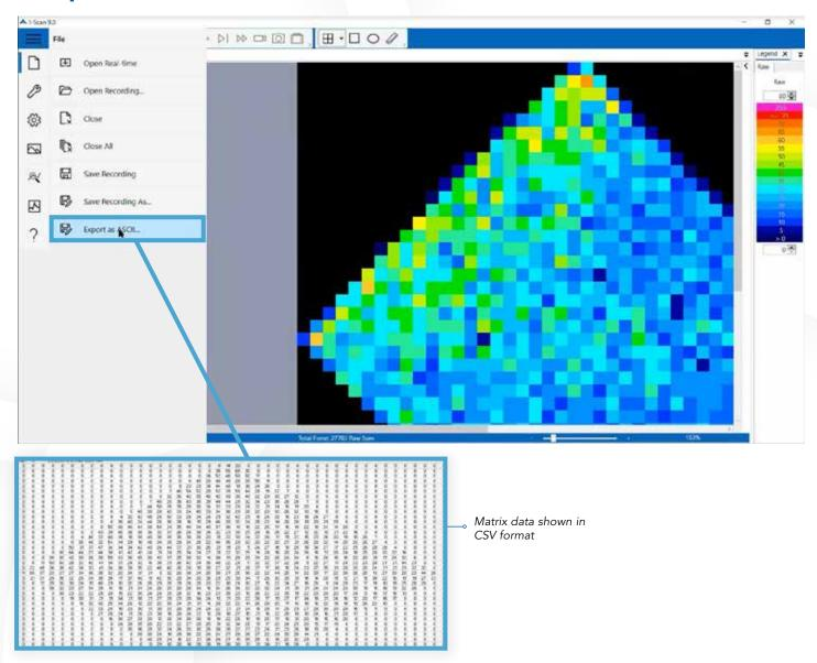
**Save as ASCII:** Save the recording pressure data in an ASCII file, so data can be exported to other software. Multiple frame sensing element information, center of force data, and graph data can be exported for customized analysis and integration with other data.
