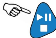
This second key can be used to switch to Leq mode and start, pause or stop acquisition.
