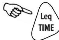
The key on the CA 1310 can be used to select the duration as required among the following values: 10 seconds, 1 minute, 5 minutes, 10 minutes, 30 minutes, 1 hour, 2 hours, 4 hours, 8 hours, 16 hours, 24 hours.
