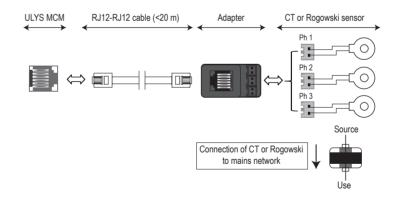
The RJ12 connection cable must be a maximum of 20 m in length and is available from Chauvin Arnoux Energy in several length variants.
