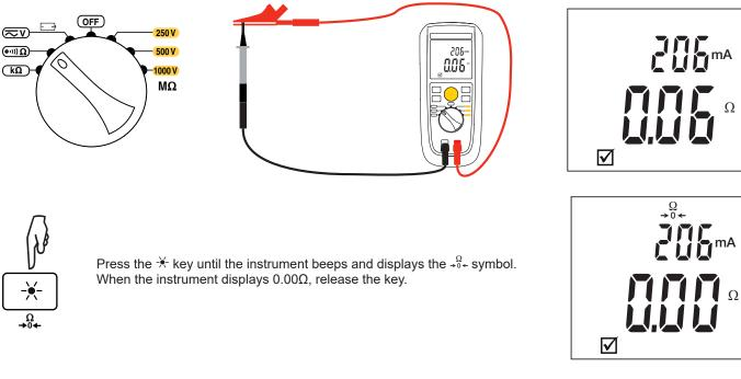
The leads are also compensated for resistance measurements. The compensation is retained even after the instrument is switched off.
