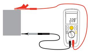
The instrument displays the AC+DC voltage. If it is >30V, the AC+DC voltage on the terminals is hazardous.
