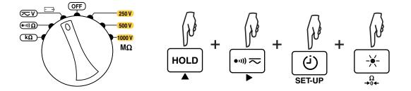
At each step, press the **TEST** key. The instrument performs the adjustment and displays the result (**PASS** or **FAIL**) Press the  $\blacktriangleright$  key to go to the next step or  $\blacktriangle$  to return to the previous step.
