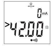
If the display unit indicates >42.00 $\Omega$ , the fuse has blown and must be replaced.
