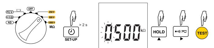
Use the  $\blacktriangle$  key to set the digit and the  $\blacktriangleright$  key to go to the next digit. When all 4 digits have been set, choose the unit. Confirm by pressing the **TEST** button.
