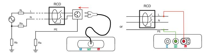
The instrument first of all checks that the voltage between the L and PE terminals is correct. If it is, the  $\frac{1}{2}$  symbol lights steadily. If not, the symbol blinks and it is not possible to make a test. If  $U_{LPE} < 90 \text{ V}$ , the instrument displays  $U_{LPE}$  and  $U_{NPE}$  in alternation.
