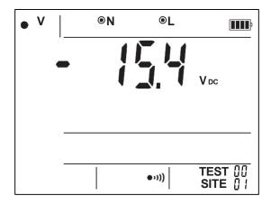
In the case of a live measurement (LOOP or RCD), the instrument shows where the phase should be on the outlet using the symbol. If the phase is on the wrong side, the for symbol blinks to indicate that the tripod cable must be reversed.
