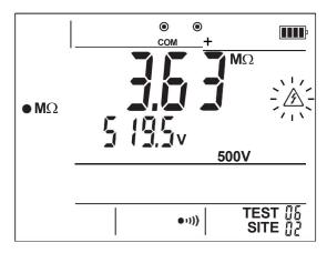
When you release the **TEST** button, the instrument displays **dIS** (discharge) to indicate that it is discharging the object tested. If the object is not capacitive, discharging is very rapid. When the voltage falls below 25V, the **dIS** and **S** symbols disappear from the display unit.
