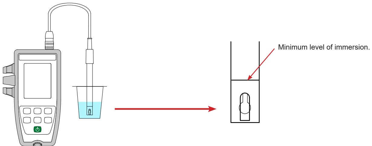
The electrode supplied with the instrument has an integrated temperature probe. There is therefore no need to measure the temperature of the solution.
