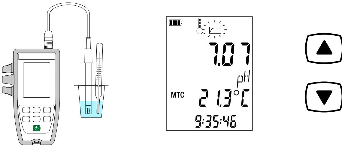
The instrument corrects the response of the electrode for temperature.
