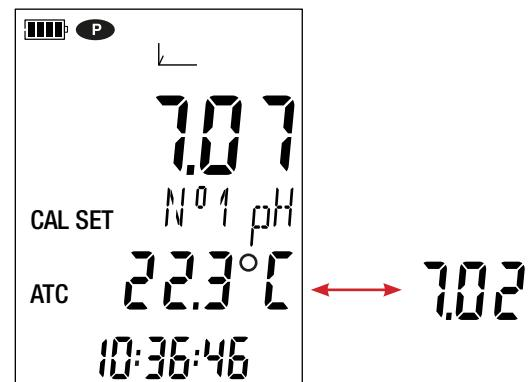
The instrument performs the pH measurement and indicates its progress.
