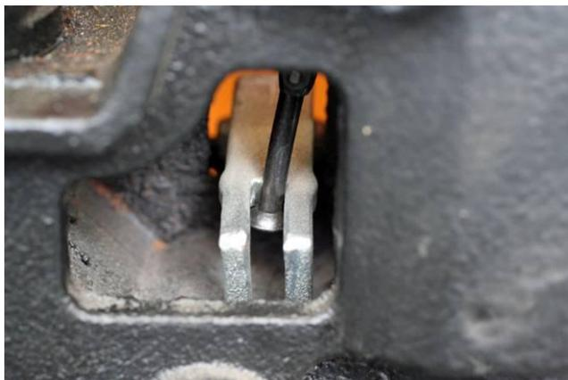
⇒ To start-up the lifting mechanism screw down the adjustment screw till to the preset stopper
