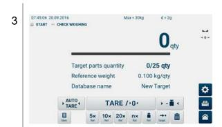
Place weighed load on the balance and start counting. The capacity indicator facilitates weighing to the nominal value. Display example see chap. 10.1.3.1
