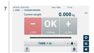
Tare, as required, place the load on the weighing pan and start tolerance control.
