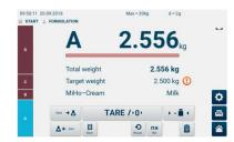
Weight of the component is over the nominal weight/tolerance
