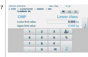
Either enter lower limit value numerically or accept loaded weight as lower limit value with
