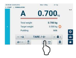
If a nominal weight is exceeded, press and the nominal weights of the other components are calculated proportionally to the exceeded weight value.
