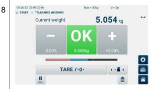
The colour of the indicators <->, <OK> and <+> changes depending on the loaded weight. You will hear a signal when the target value has been reached.
