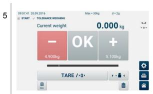
Tare, as required, place the load on the weighing pan and start tolerance control. The indicators <->, <OK>. < + > and the capacity indicator show the sample weight in relation to the tolerance limits.
