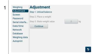
Unload the balance. Ensure that there are no objects on the weighing pan. Tap <Continue>.
