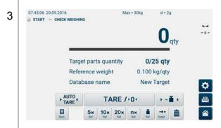
Place weighed load on the balance and start counting. The capacity indicator facilitates weighing to the nominal value.
