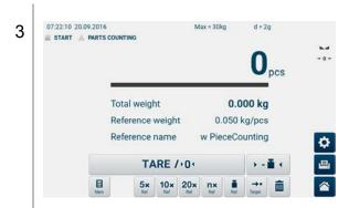
The reference item weight is displayed. The balance is now in parts counting mode counting all units on the weighing pan.
