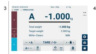
The balance is ready for weighing the first component. Displays the name and the nominal weight.
