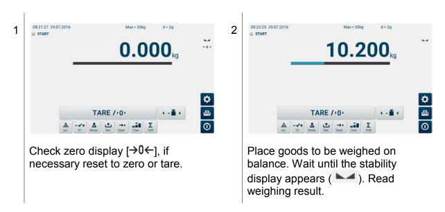
Depending on the setting in <Technical setup → Autoprint activated/deactivated> the weighing value can be output either automatically by connecting an optional printer or after tapping .
