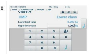
Either enter upper limit value numerically or accept loaded weight as upper limit value with
