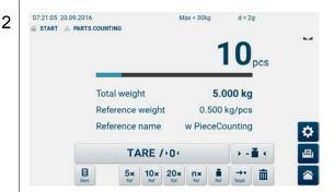
Tap on loaded reference item quantity (e.g. 10x ). The balance determines the weight of the reference item.
