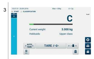
Load the article. The class will be shown according to the loaded weight. If an optional printer has been connected, a measurement protocol is printed (depending on the setting in the menu either
