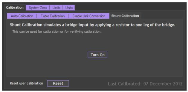
Click the 'Turn On' / 'Turn Off' button to toggle the shunt calibration output. The shunt cal internally connects a resistor across the strain gauge bridge. This causes a change in value that can be seen on the Information page
