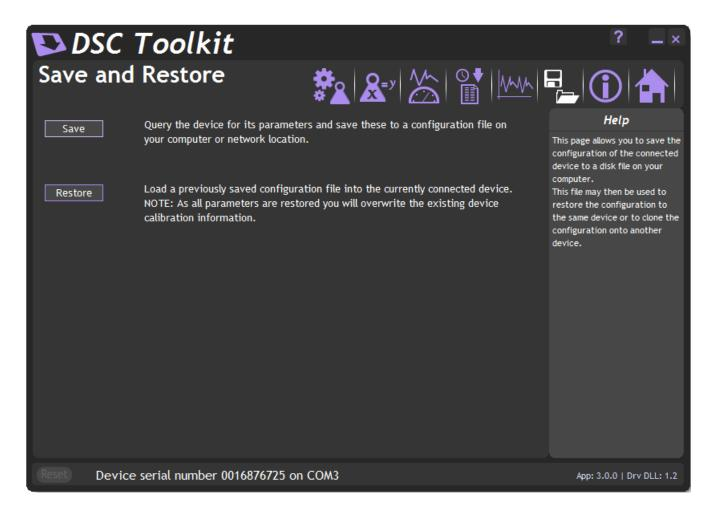
Clicking the 'Save' buttons will allow you to specify a file to which the configuration of the connected module is written.
