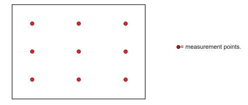
Place the sensor on the first measurement point and press the **MEM** key to record the value in memory. The counter is incremented. Proceed in the same way for all the other points of the map.
