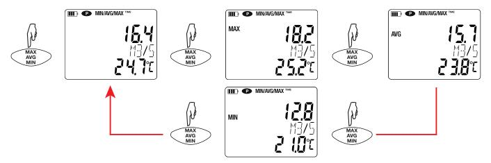
To exit from the MAX AVG MIN mode, long-press the MAX AVG MIN key.
