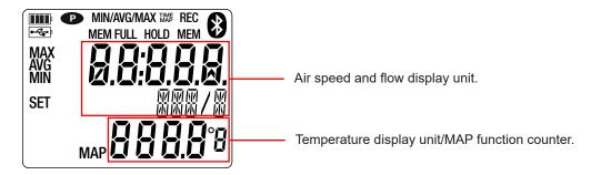
When the measurement exceeds the limits, the instrument displays OL.
