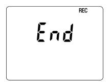
If during start-up the instrument displays the screen shown opposite, it means that a recording session has been brutally interrupted by a power outage.
