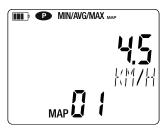
When all of the points have been entered, you can look up the maximum, the mean, and the minimum of the values entered. To do this, press the MAX AVG MIN key 3 times.
