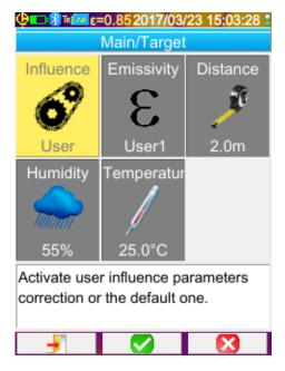
When user compensation is selected, the various parameters can be adjusted:
