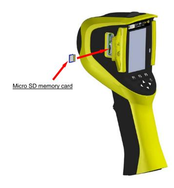
The files created by the camera (image, audio, and setup files) are stored only on the micro SD memory card located on the left side of the head.
