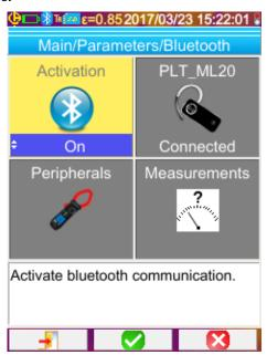
To use this function, you must first activate it from the Main/Parameters/Bluetooth menu by setting the Activation item to "On" (validate the item with **F2** , to allow entry, use Up/Down to change the value, and **F2** to validate the
