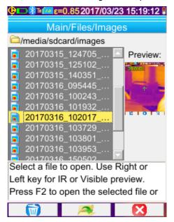
The file manager lists only infrared images generated by the camera bearing a name in the form
