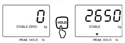
The peak load will be held on the display until deleted by pressing For that, press for about 2-3 seconds. The ▼ above **PEAK** disappears.
