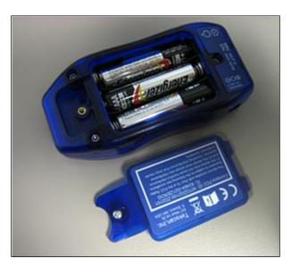
4. Place the battery access door back onto the Transmitter. Insert and screw the battery access door in place. As you tighten the screw, be careful not to strip the threads.
