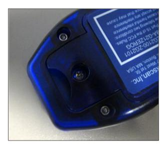
2. Lift and remove the battery access door using the thumb notch to reveal the batteries inside the Transmitter. Replace the three AAA batteries with a new set.
