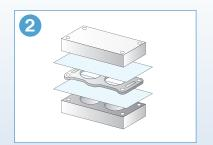
Insert Prescale between the pressure surfaces to be measured.
