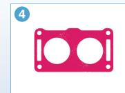
Remove Pressure and Prescale and you can now see and check the pressure and its distribution.
