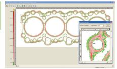
The specified field is enlarged. (x4,x8,x16) Pin point pressure values can be displayed on the image.
