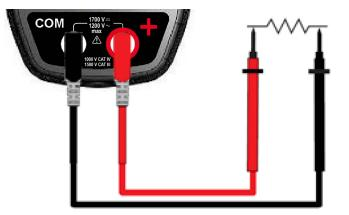
An audible signal is emitted if there is continuity, and the measured value is displayed on the screen.
