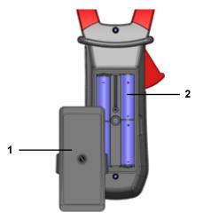
Figure 6: the battery compartment cover
