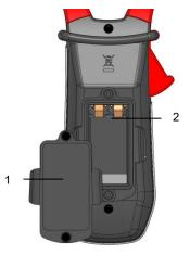
Figure 6: the battery compartment cover
