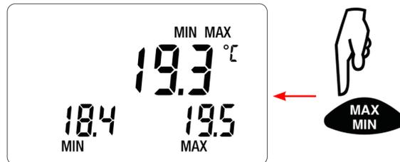
Display of MIN MAX in temperature
