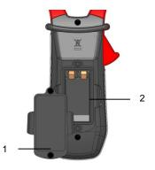
Figure 6 : the battery compartment cover
