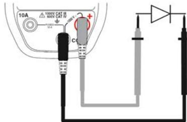
5. Read the junction threshold voltage measurement indicated on the display.
