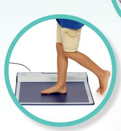
Pressure measurement mat for quick and portable balance, foot and gait assessments.
