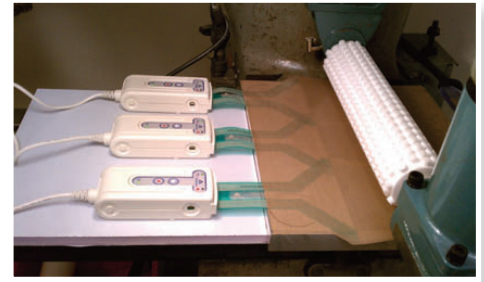
PVA Brush Roller over Pressure Mapping Sensors
