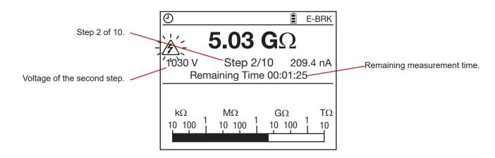
You can view the graphical representation of the measurement results by pressing the GRAPH key. For more details, refer to § 4.5.
