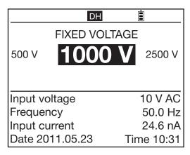
Setting to High is recommended when you make measurements in the presence of strong electromagnetic fields at the network frequency (for example near high-voltage lines).
