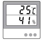
This measurement varies greatly with the temperature and the relative humidity. It is therefore essential to measure them using a separate device (see §1.2) and to record them with the insulation value.
