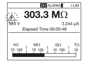
This function is useful in case of high instability of the insulation values displayed, but it is also possible to estimate the measurement on the bargraph.
