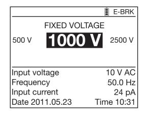
The measurement will be stopped when the current reaches the maximum value (Maximum Output Current) defined by the user (see below). This type of test is useful for testing variators or other types of voltage limiter. The I-LIM symbol is displayed.
