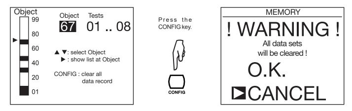
The instrument in this case completely reformats the memory, which takes a few minutes. During this time, it displays WAIT.
