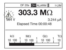
fluctuating high insulation resistance values. Such fluctuations may be due to hand effects, fluctuating capacitances in the device tested, insulation that varies because of conducting dust, an ionizing and polarizing effect of this dust, etc., or again to the presence of an AC voltage superposed on the measurement.
