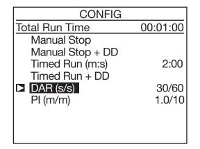
Press CONFIG to exit from the configuration menu. DAR or PI is displayed in the top left corner of the display unit to indicate the configuration chosen.
