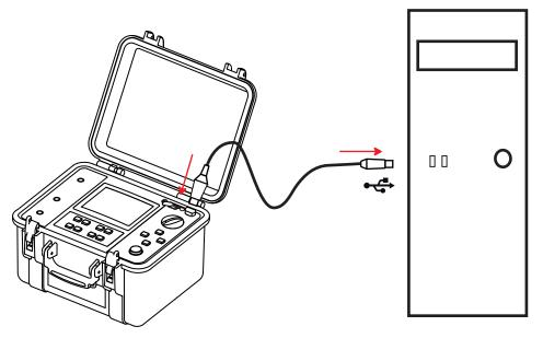
When in communication with a PC, the instrument displays REMOTE and no longer reacts to the user's commands. The keys and the rotary switch are inactive, except for stopping the instrument (OFF setting). To use the data transfer software, refer to the on-line help.
