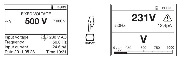
When the external voltage exceeds 25V, the blinking ( A) symbol is displayed alongside it.
