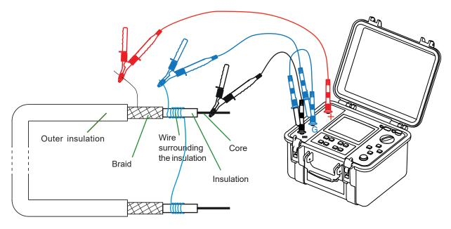
Using the guard eliminates the influence of the surface leakage current. A conducting wire must be wrapped round the insulation.
