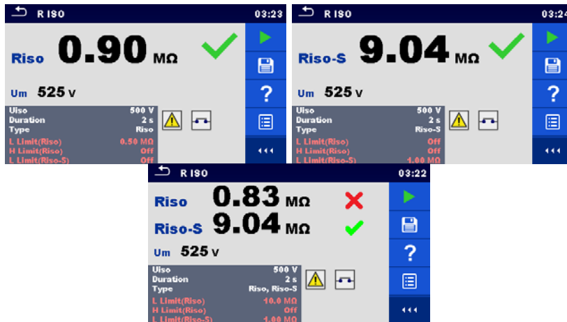
Figure 4.27: Examples of Insulation resistance measurement results
