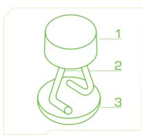
The end of the sensor's body (1), the thermocouple fins (2) are brazed onto a tip (3).
