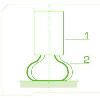
At the end of the sensor's body (1), the thermocouple fins (2) are soldered and guarantee proper application of the hot point to the surface. Some models marketed with the "surface sensors" description give errors that can be more than 20 °C at high temperature (300 °C). Below is an example of a contact-type surface temperature sensor that is not suitable for measurement purposes\*\*:
