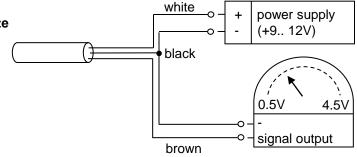
B) This circuit is recommended for **relative** torque measurement e. g. 0 V equals to approx. 0 Nm.
